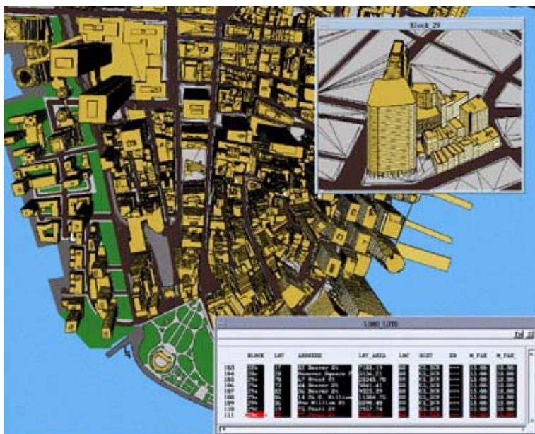
Fig. 3. Lower Manhattan Three Dimensional Geographic Information System (3D/GIS): developed to analyze policy and planning scenarios for the revitalization of Lower Manhattan. (Environmental Simulation Center)
